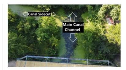
A sidecut is like a small "driveway" off the main canal. Entrepreneurs could use private funding to build a sidecut for efficiency and direct canal access. The sidecut pictured above, used by Spears, Case & Co., is still easily seen from the VanScoy Towpath Trail near the foot of Main Street in Delphi.
